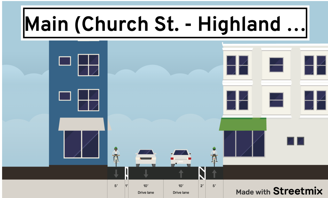
Figure 12: Segment 2A Main from Church St. to Highland Ave.
