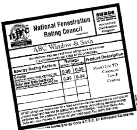
▲ Example of a manufacturer’s NFRC label showing the window U-factor (called the “U-Factor” here).
