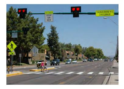
Typical installation of Pedestrian Hybrid Beacon
