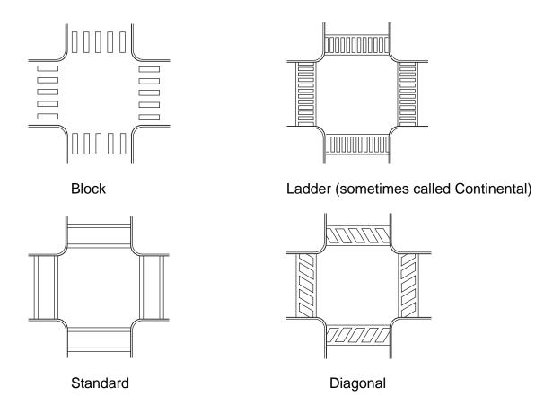
Figure 9: Allowable crosswalk marking patterns
