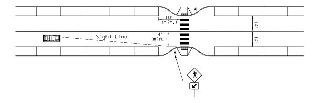
Figure 14: Mid-block Bulbout Example
