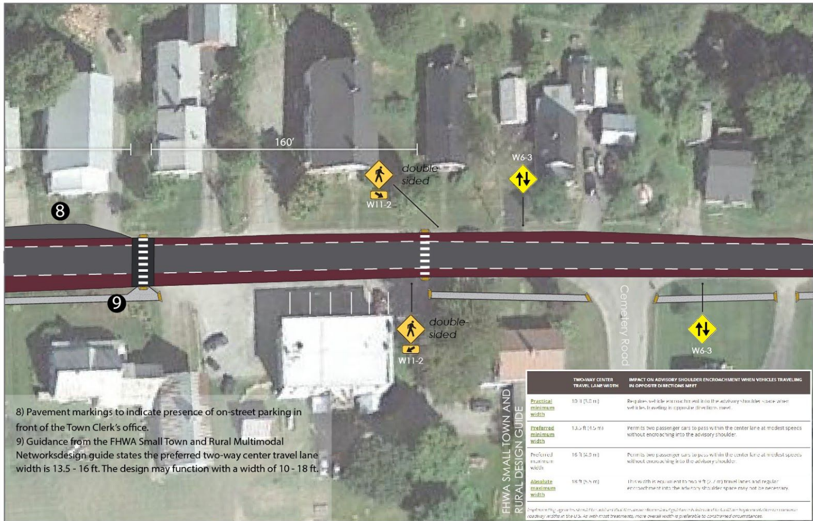
Figure 5g. Two-Way “Slow Street” Design with Advisory Shoulders for Pedestrians and Bikes at E. Craftsbury Rd
